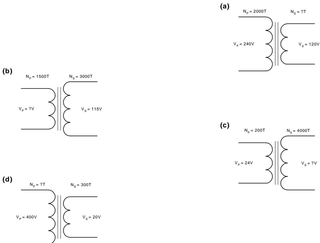
For each of the examples above, state the transformation ratio and whether the transformer is step up or step down :
