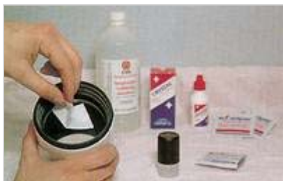
One convenient lens cleaner is the E-wipe, a lint-free pad soaked with methanol. You drape the wipe on the glass, pull it across once, and discard. The methanol dries in moments, leaving a clean surface free of dirt, oils, or grease. S&T / Chuck Baker
