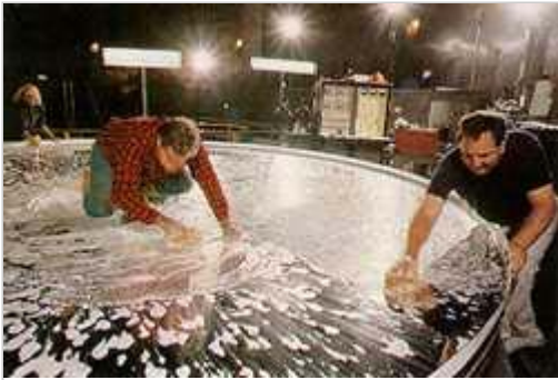
Big-time optical cleaning. The primary mirror for the 200-inch telescope on Palomar Mountain is washed (with special material) and realuminized every two or three years. Roger Ressmeyer / © Corbis
