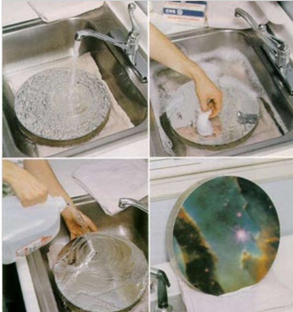
Washing a 12-inch telescope mirror. The safest way to remove grit is to blast the surface with tap water. That may be all you need to do. If dirt remains, swish the surface very lightly with clean cotton in lukewarm water and detergent. Rinse with tap water, do a final rinse with distilled water, and set up on edge to dry. Sky & Telescope / Chuck Baker
